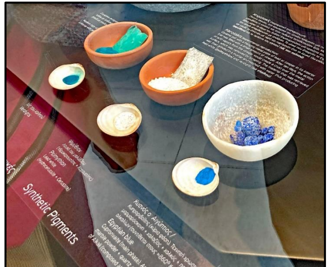
Synthetic pigments, including (right to left) Egyptian Blue (Cuprorivaite, calcium copper silicate, when natural), and Lead White (Hydrocerussite and Cerussite when natural), and Verdigris (copper acetate).
