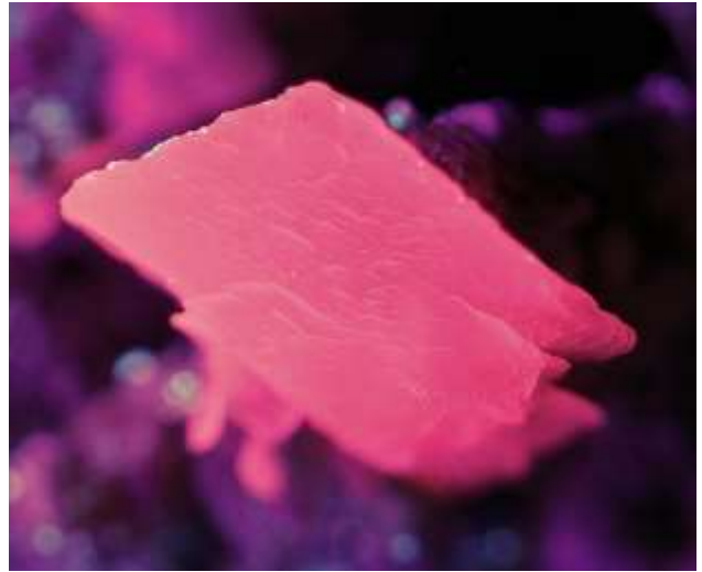
Calcite crystal on Ferberite specimen above, illuminated with short-wave ultraviolet light. Stack of 12 photos taken with 60 mm macro lens. FOV 12 mm.
